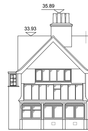
8 ELEVATION SOUTH ELEVATION - COTTAGE 1 : 200
